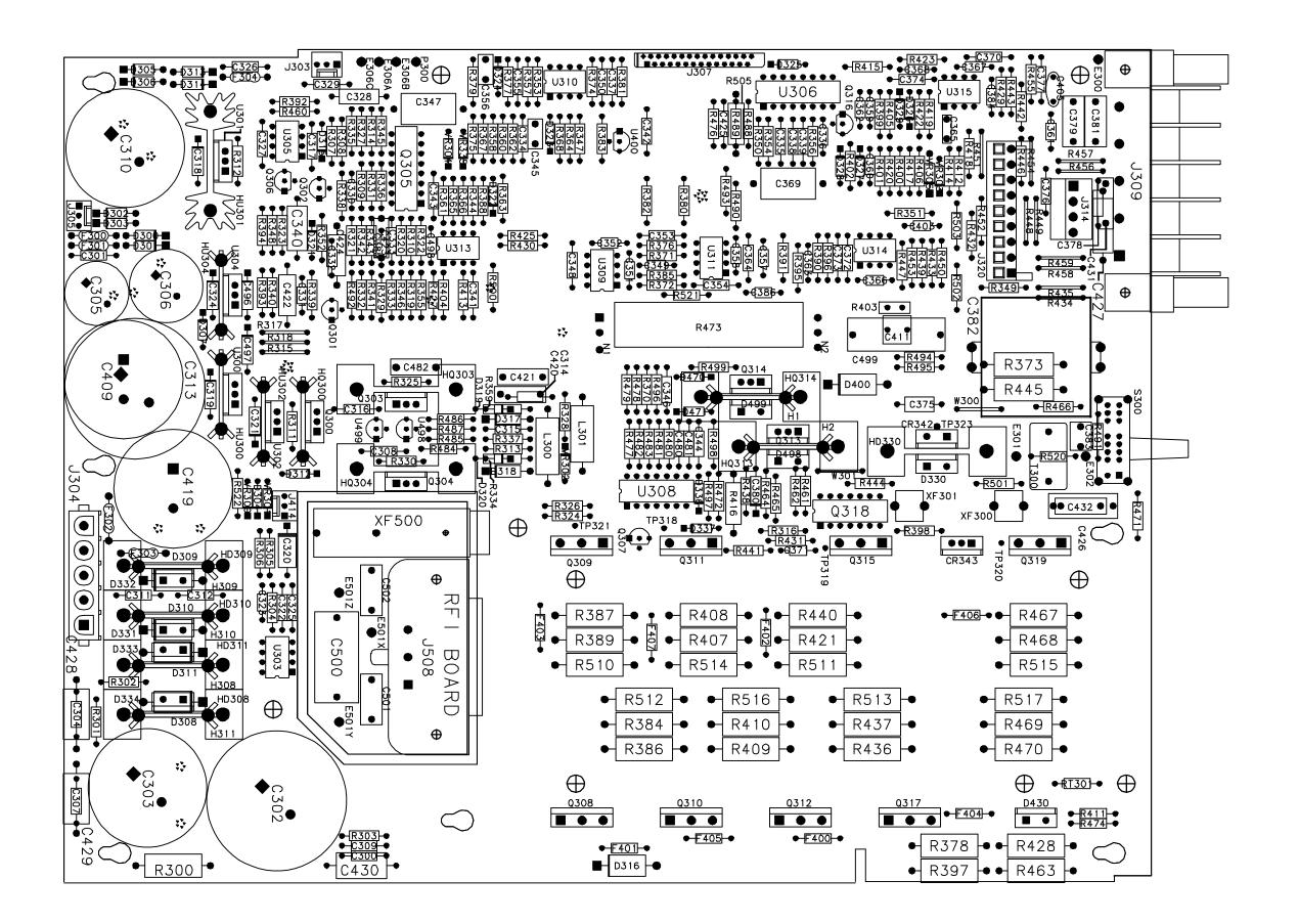
Figure 6-1. A1 Board Component Locations
