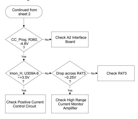
Figure 3-1 Sheet 10. No Current Limit
