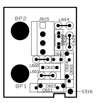
Figure 6-2. A4 and A6 Board Component Locations
